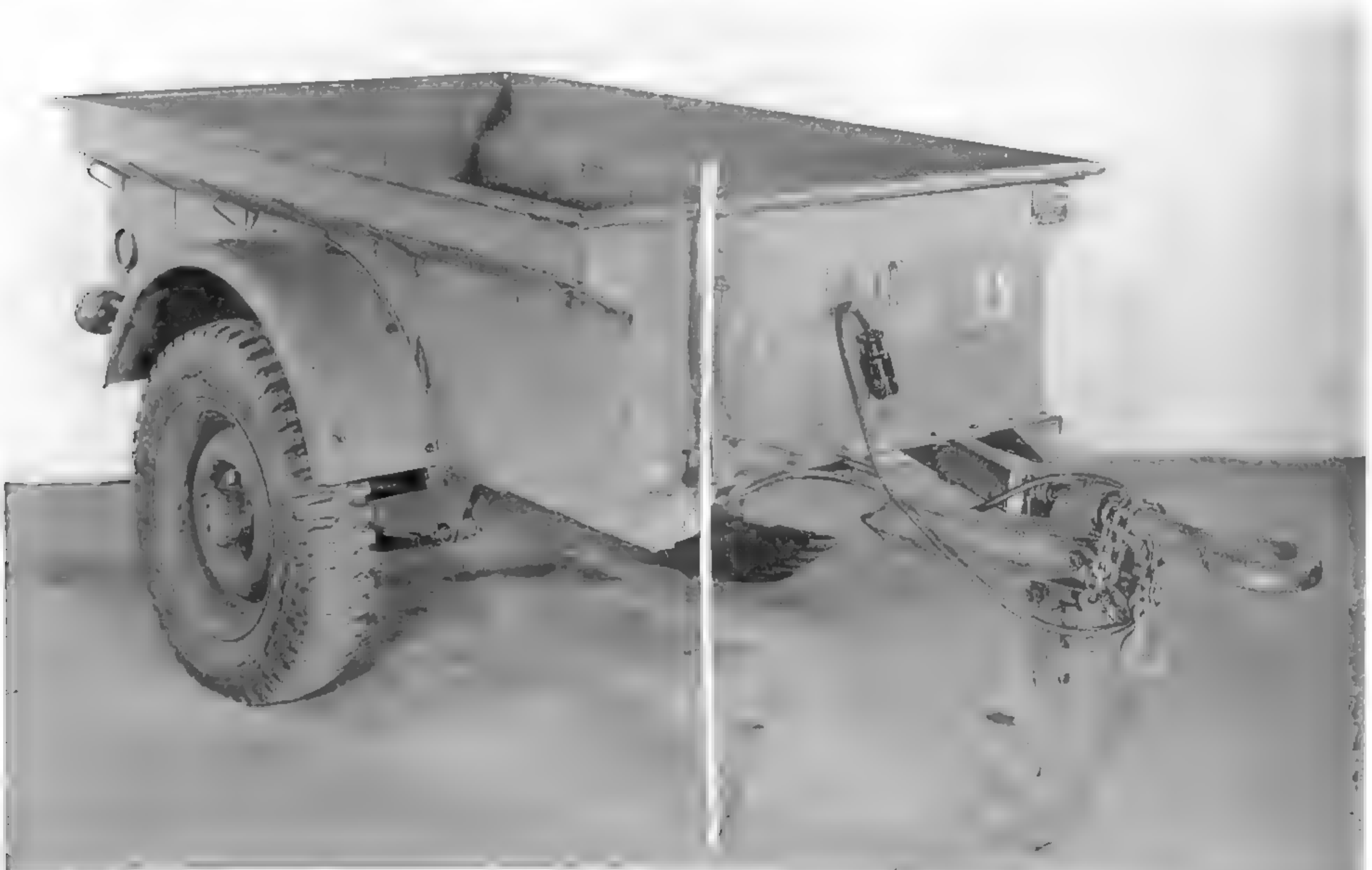
Willys also produced a 1/4-ton trailer, using bodies supplied by Central Manufacturing. The axle of the Willys trailer differed from that used on the Bantam-built product. (U.S. Army photo)
